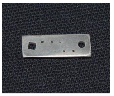
Sample of a metal part printed using the Prodways© R&D technology
